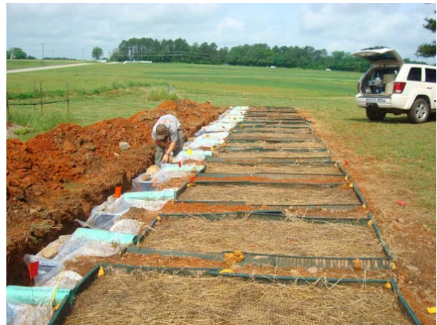
Figure 1. Site 1 immediately after installation. Plastic sheeting over runoff containers kept out rain.
