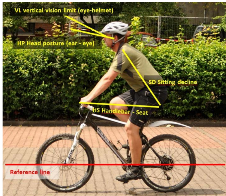
Figure 1. Establishment of angles relevant for seating geometry and vision limits.
