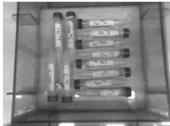
Figure 3. MAGICA calibration tubes arrangement in the water phantom.
