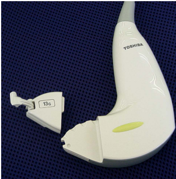
Figure 1. The PVT-350BTP supports four puncture angles: 55 degrees, 70 degrees, 85 degrees, and 100 degrees. It has only one needle slot, but 13 G to 22 G needles can be used by adjusting the screw.
