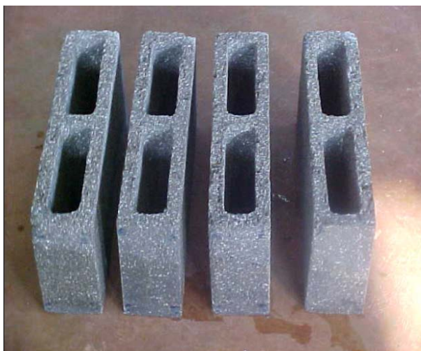
Figure 6. Application of Portland cement mortar-eggshell particles.
