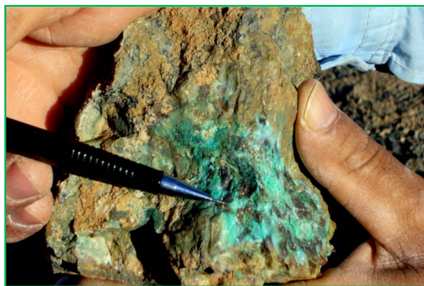
Figure 3. Sulphide mineralization (chalcopyrite and pyrite) in basalt that has been converted into iron hydroxides, chalcocites and covellite by the supergene processes.
