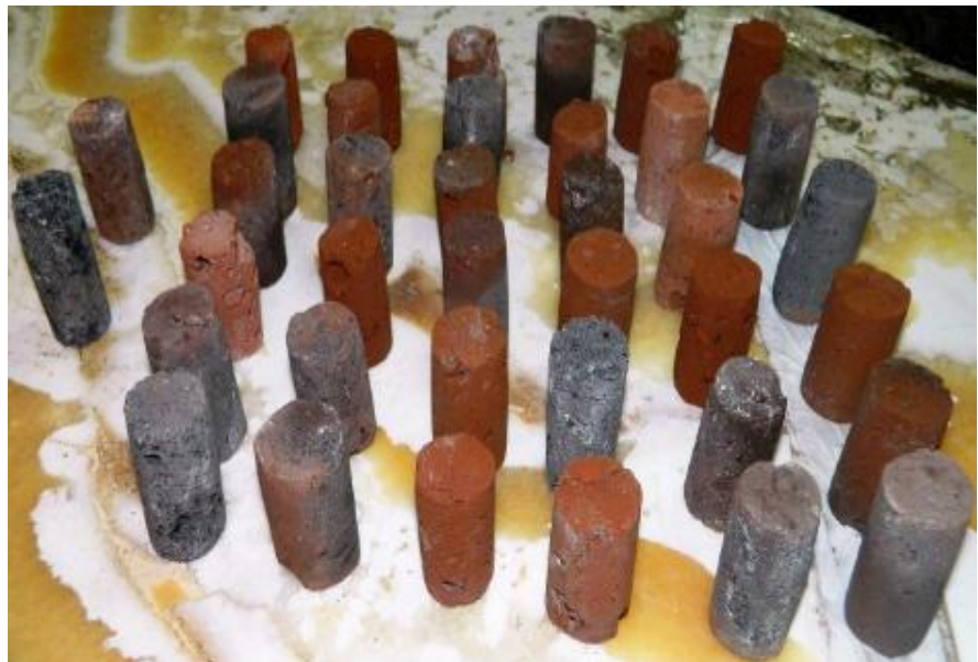
Figure 14. Investigated roman and byzantine bricks cylindrical specimens. Different colors and textures are obvious.
