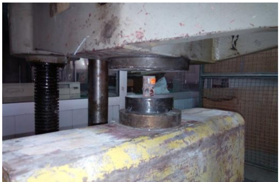
Figure 22. Uniaxial compression test on the brick cylinder samples.
