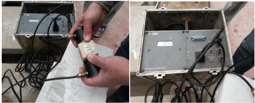
Figure 23. Non-destructive Ultrasonic pulse testing.
