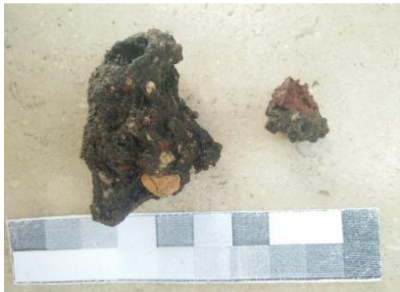
Figure 33. Mortar sample after etching by dilute HCL, Note that: limestone, brick and furnace slag fractions are detected.
