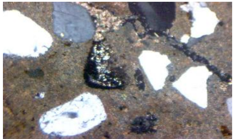
Figure 31. Microscopic photograph showing aggregates of lime and ceramic brick together with quartz grains (C.N, sample M2).
