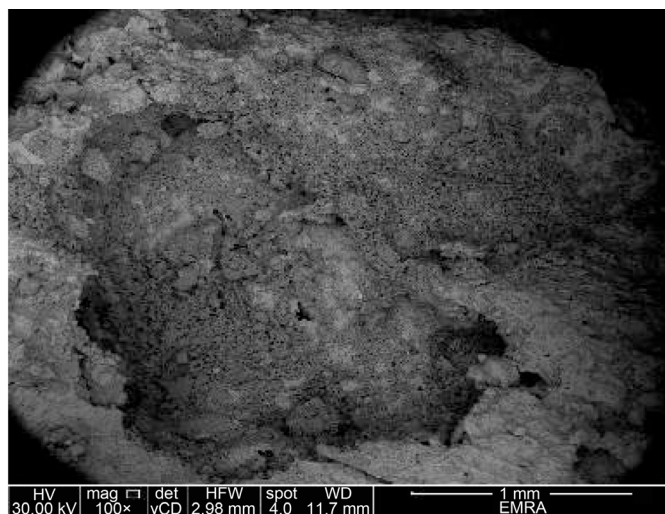
Figure 38. SEM image showing the brick aggregate fractures inside the mortar sample.
