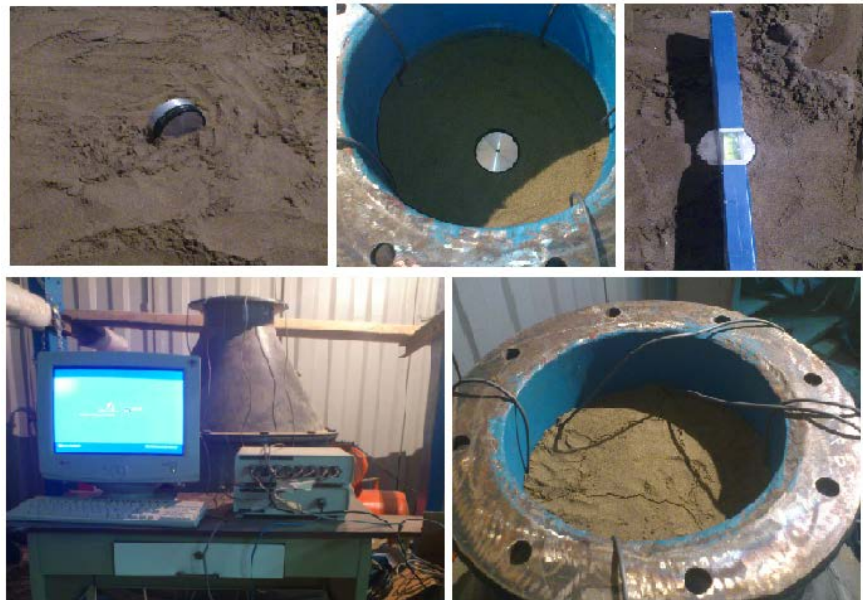
Figure 9. Sensors for studying vertical and horizontal stress distribution in FCV-AUT.
