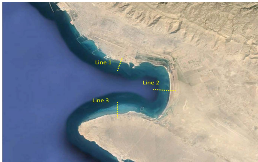
Figure 8. Positions of lines perpendicular to the coast to calculate longshore sediment transport rate.
