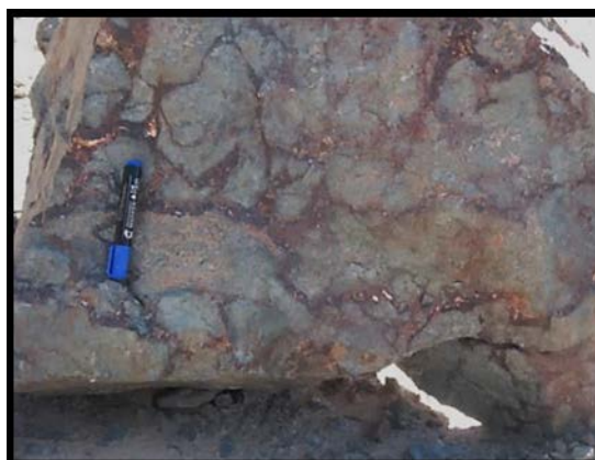
Figure 4. The breccias consist of angular fragments of the metasomatic host rocks cemented by iron ore.
