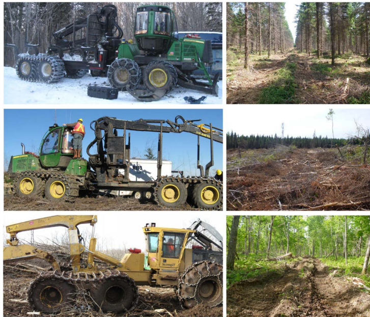
Figure 2. Left; wood-forwarding equipment: JD 1110E (top), JD 1510E (middle), and TC 635D (bottom). Right; wood harvesting-forwarding operations: commercial thinning (white spruce plantation, top), clearcutting (middle), hardwood shelter-wood cutting (bottom).
