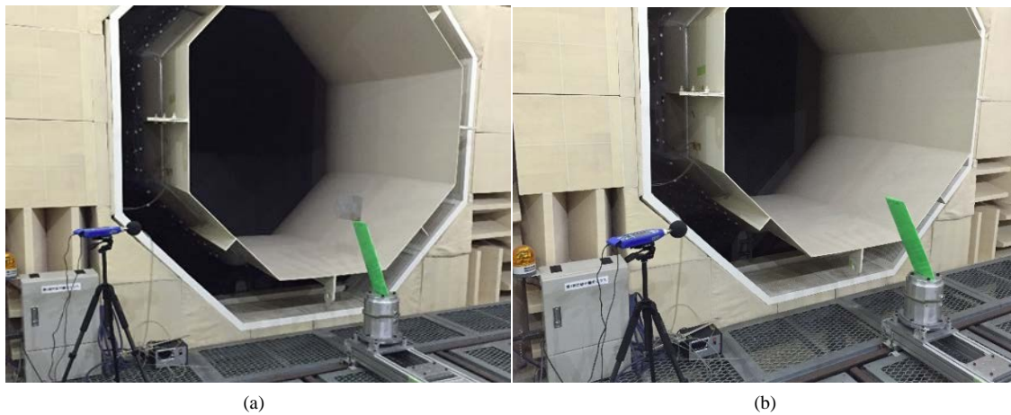
Figure 9. Measurement of aerodynamic sound radiated from the delta wings in low-noise wind tunnel. (a) Measurements of aerodynamic sound; (b) Measurements of background noise without delta wings.
