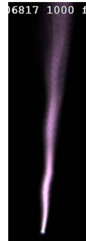
Figure 5. Corona discharge starting from top of the central cone of dynamic emitter. One can see spiral structure in the violet luminous part of the jet. Pre-chamber pressure was 8·atm. Here shutter speed was 1000 frames per seconds. Corona discharge was provided to obtain the spectra.
