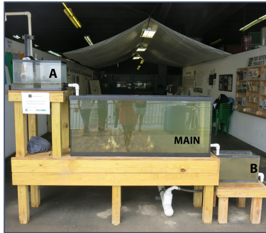
Figure 1. The River Project living oyster reef. Tank A receives the initial flow of HRE water, which spills into the Main Tank and returns to the Hudson River by Tank B (Photograph by J. Perrino).
