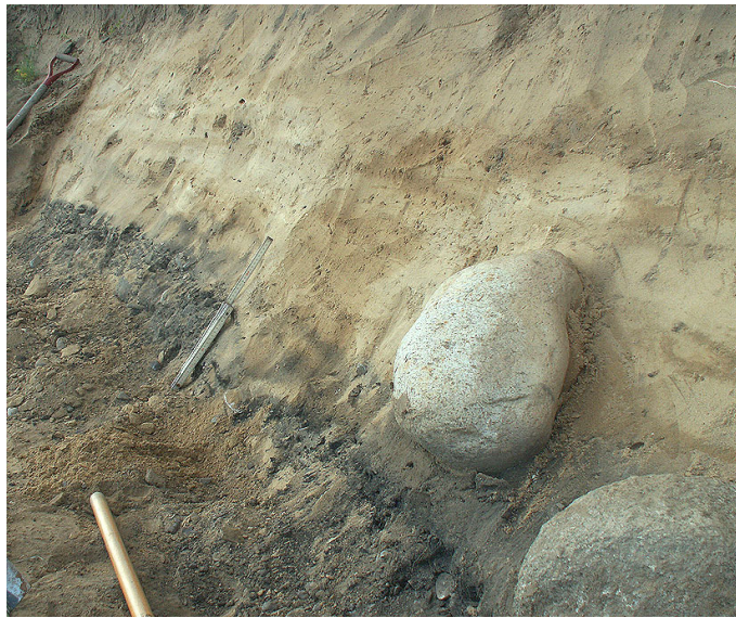
Figure 17. The black land surface (layer 2 in Figure 16) is covered by an irregular, partly liquefied, layer of humic sand (layer 3), in which the blocks rest. This layer contains reworked material (Figure 18) and constitutes a seismite of shaken and slid material.
