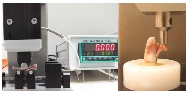
Figure 3. Example of three-point femur fracture with a measured pressure and femoral neck fracture.
