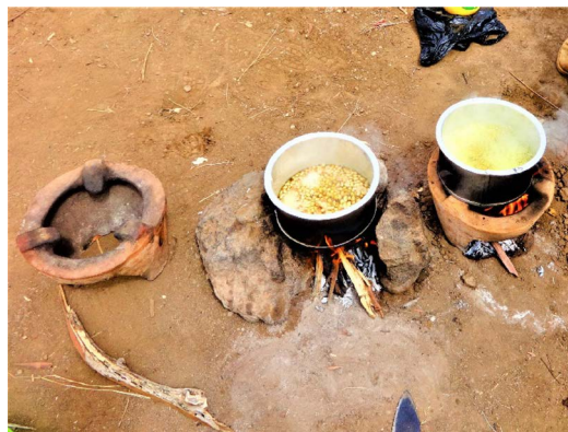
Figure 2. Left energy saving stoves liner, Middle-traditional open fire, and Right-energy saving stoves with fire.
