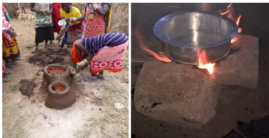
Figure 1. Left: Amboseli women group installing a model energy saving stoves during the training session, and Right: three stone traditional open fire set up.
