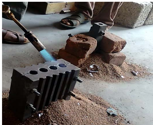
Figure 2. Pre-heating of mould box.
