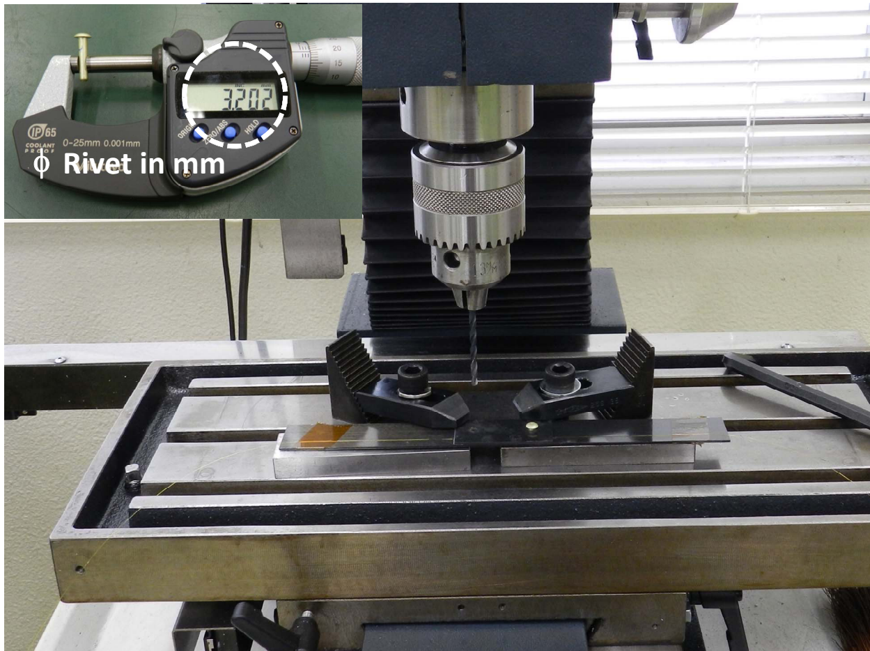
Figure 5. Drilling process and rivet installation.
