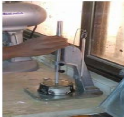
Figure 6. Vicat device with 10 mm diameter probe.
