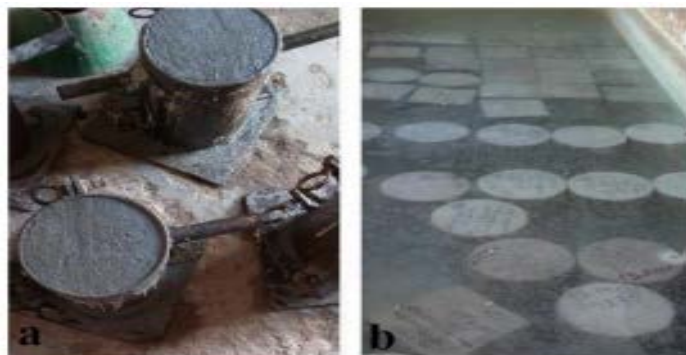
Figure 9. 16 cm × 32 cm mold and concrete curing tray.
