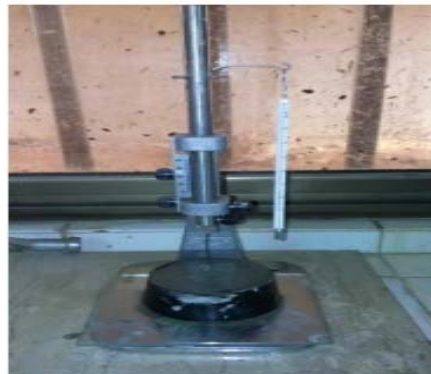
Figure 7. Vicat apparatus equipped with a 1.13 mm needle for the setting test.
