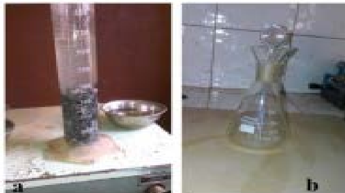
Figure 5. Graduated cylinder and pycnometer for the measurement of specific gravity.
