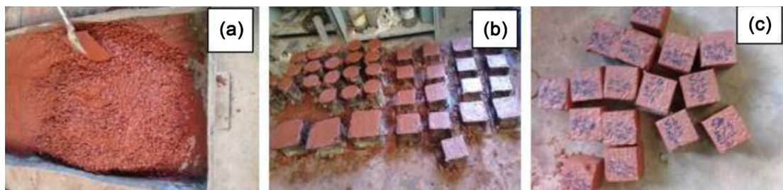
Figure 3. Preparation of samples (a) mixing (b) casting and (c) demolding.
