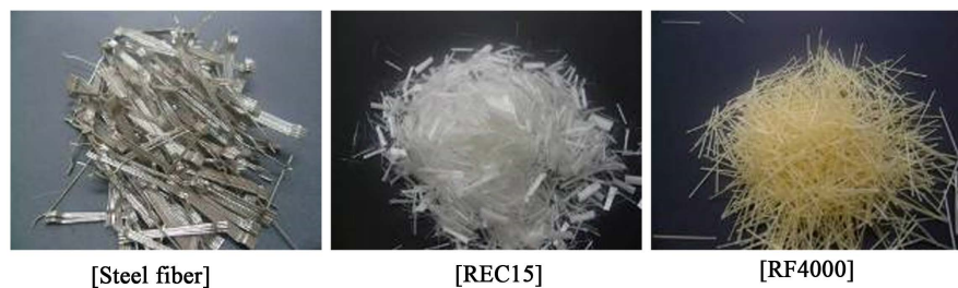
Figure 2. Shapes of steel and PVA fiber.
