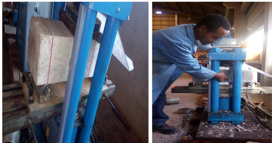
Figure 5. Flexural strength test in the laboratory.
