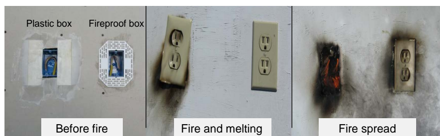
Figure 3. Stages of fire spread from wall plug (Courtesy of BPMI, Inc. ( http://www.bpmi-usa.com/ ) [25]).
