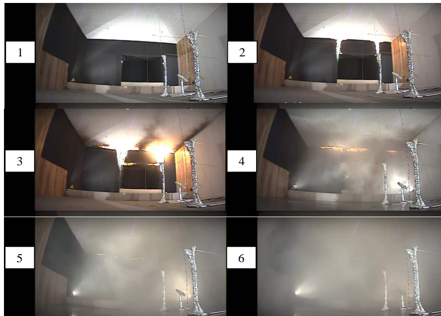
Figure 4. Activated sprinkler in a fire test to replicate the station nightclub fire (Courtesy of National Institute of Standards (NIST): https://www.nist.gov/sites/default/files/documents/el/disasterstudies/ncst/Final_RI_Station_Nightclub_Status_12-3.pdf [27]).
