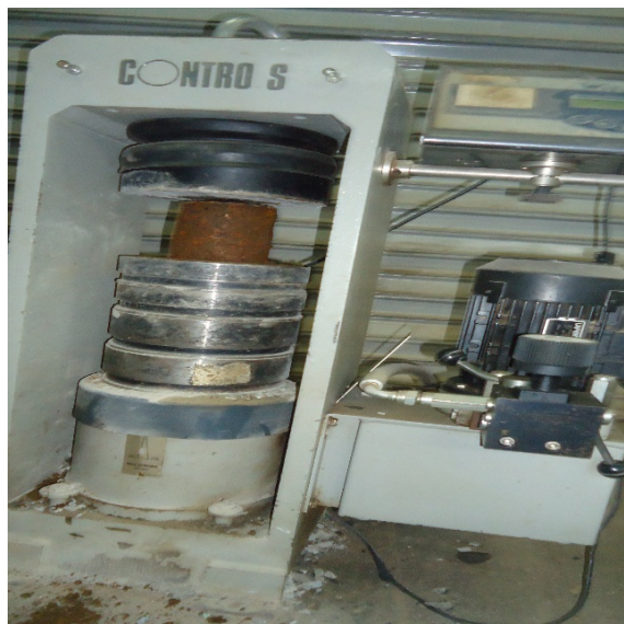
Figure 2. Compressive strength testing at MTRD on a core.
