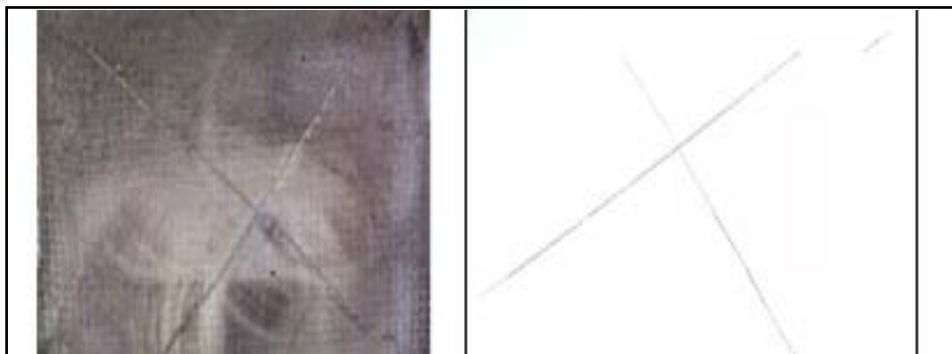
Figure 6. “X” cut on reinforced polyester with fiberglass and epoxy coating. Reinforced polyester with fiberglass (a); Epoxy coating (b).
