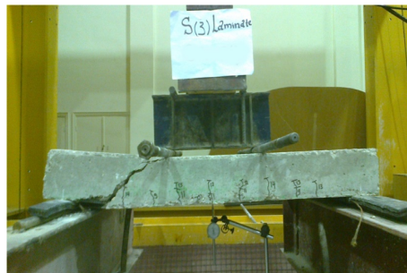
Figure 10. Test setup & crack pattern-specimen (S3).
