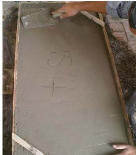
Figure 3. Final casted specimen.
