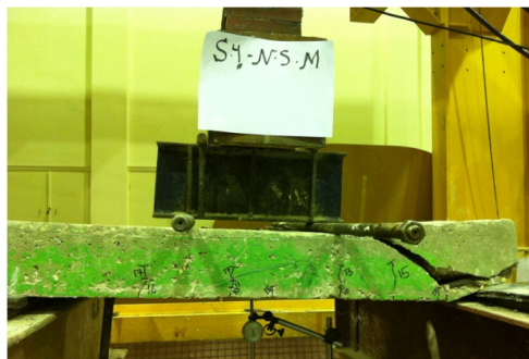
Figure 11. Test setup & crack pattern-specimen (S4).
