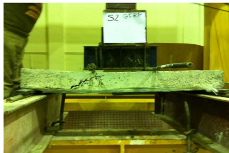
Figure 9. Test setup & crack pattern-specimen (S2).
