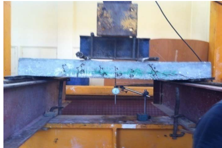
Figure 8. Test setup & crack pattern-specimen (S1).
