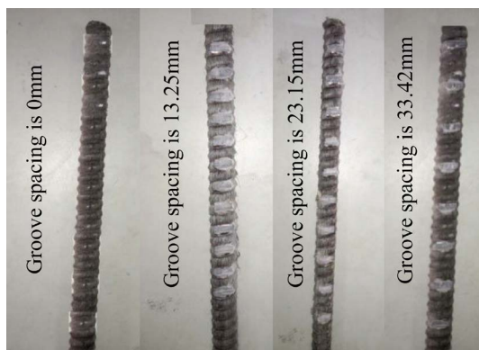
Figure 2. Test-pieces different on groove spacing.
