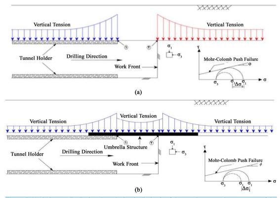
**Figure 2.** Vertical stress distribution along the longitudinal axis of the tunnel crown and stress on top of the drilling profile. (a) Not using the umbrella method; (b) Using the umbrella method.
