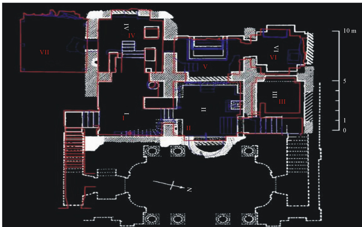
Figure 6. Digital overlay of the crypt in the basilica of Santa Maria in Via Lata detected three-dimensionally (in red section, projections in blue) with graphs of planimetric Richard Krautheimer (in white), from KRAUTHEIMER—CORBETT—FRANKL 1971.
