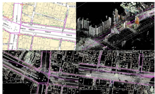
Figure 7. Taipei street excavation map [17] and the overlapping of the point cloud model with the street excavation map.
