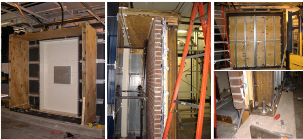
Figure 5. Wind loading test setup.
