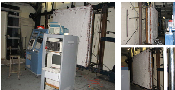
Figure 6. Racking test load facility (DRTF).
