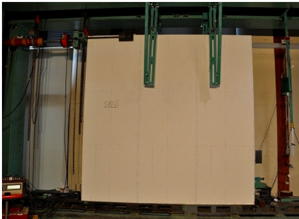
Figure 9. Test set-up for shear wall with out opening (SW).
