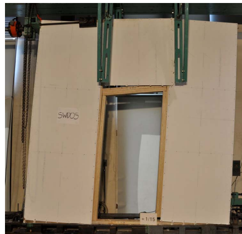
Figure 24. Final condition of shear wall with window type opening (SWWOS).opening (SWWOS).
