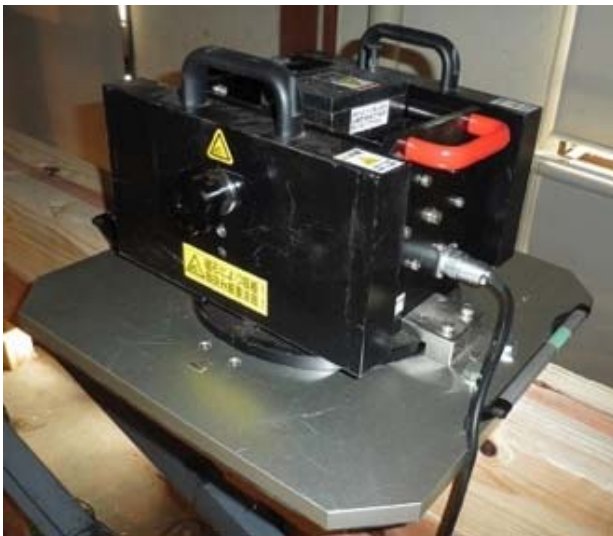
Figure 10. The portable shake excitation machine.
