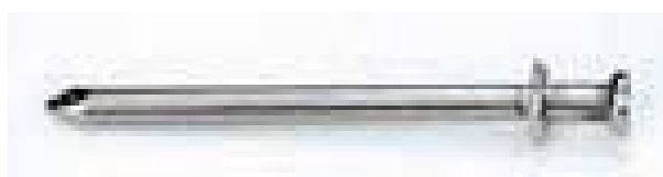
Figure 3. The steel nail used as fastener between sheathing and frame member.
