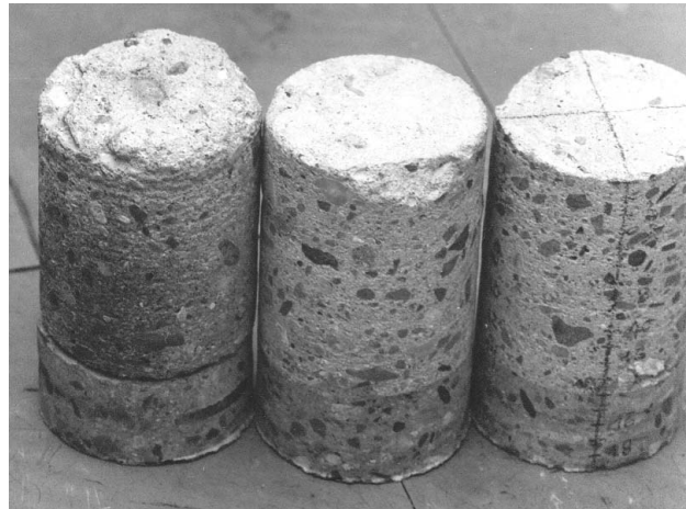
Figure 10. Macroscopic examination shows more porous structure in upper zone of concrete in cores.
