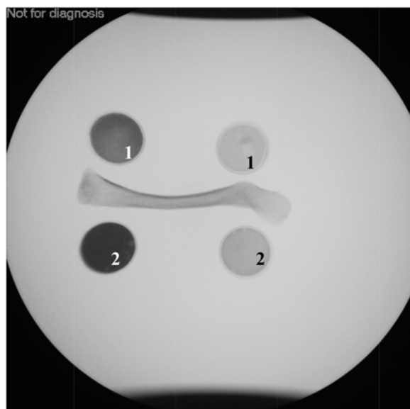
Figure 2. Radiograph of samples 1 and 2 with 1 cm (light) and 2 cm (dark) thicknesses, with a clavicle as control.
