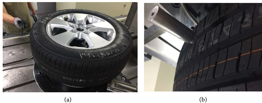
Figure 2. Tire-cavity-wheel impact test setup. (a) Test setup (fixed); (b) Impact hammer.
