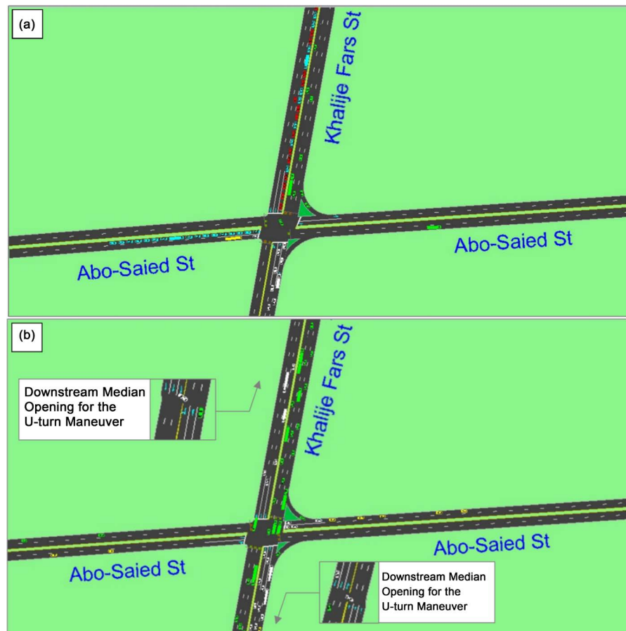
Figure 4. Simulated Study Area in SimTraffic: (A) Before Access Management, (B) After Access Management.
