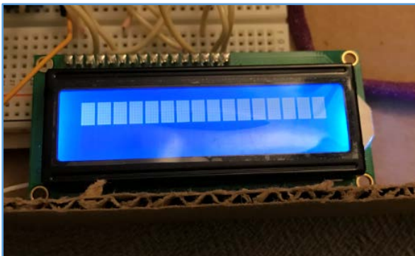
Figure 41. LCD module under test.
