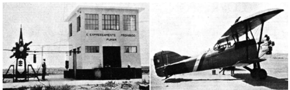
Figure 5. View of the torque-reaction test bench of the Bristol “ Jupiter ” engines built in Portugal under license (at Alverca); a Potez XXV airplane with a “ Jupiter ” engine—both entirely constructed in the Alverca workshops [12].
