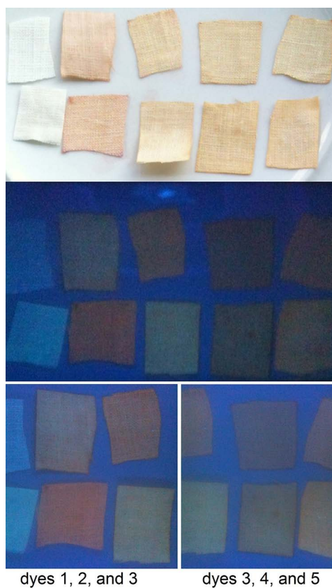
Figure S21. Ten pieces of oxygen-bleached linen dyed with different madder extracts. Five pieces in top rows: not-starched linen; five pieces in bottom rows: starched linen. Dyes from left to right, in both rows: 1. no dye, 2. root powder stirred in water at room temperature for 2 h, then filtered, then acidified, 3. root powder stirred in hot water for ca. 45 min, then filtered, then acidified, 4. root powder extracted as tea with boiling water, then spontaneously fermented, then acidified, 5. root powder extracted as tea with boiling water then acidified and stored. All dyes had a \text{pH} \leq 4 . All fluorescence photos taken through 2.5 mm thick L-42 UV-filter (Hoya), no filter in front of Wood lamp ( \sim 365\text{ nm} ). Two bottom photos: left part and right part of the rows, photographed from smaller distances. ©A.A.M. v.d. Hoeven.
