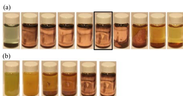
Figure 1. Plating quality with varying ascorbic acid content/pH (a) Finding the right plating in the copper after 168 hrs. Start on the left increasing amounts of 0.5 mL L-ascorbic acid was added to 10 mL of an Ammonium hydroxide/Copper sulfate solution mixed to a mole ratio of \text{NH}_4/\text{Cu} = 7.12 . From left to right: 1, 2.5, 4, 5.5, 7 (pH 8.9), 8.5 (pH 8.5), 10 (pH 7.5), 11.5, 13, 15 mL of L-ascorbic acid were added to solution and deionized water was used to raise the volume to 20 mL. On visual inspection, the best the condition was found to be 8.5 mL of L-ascorbic acid with a pH 8.5. The best sample is indicated by a black box around the sample. (b) Time elapsed observation of the optimal condition (8.5 mL of ascorbic acid) (left to right) 5 min., 1 hr, 4.5 hr, 7.5 hr, 28 hr, 168 hr.
