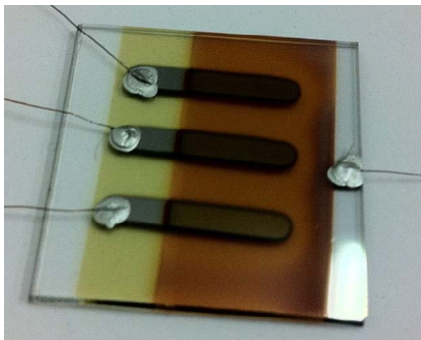
Diagram 1. Typical structure of an organic solar cell (ITO/MoO 3 -CuI/BrTPP(Zn) (4-Bromophenyl zinc porphyrin)/C 60 /Al).
