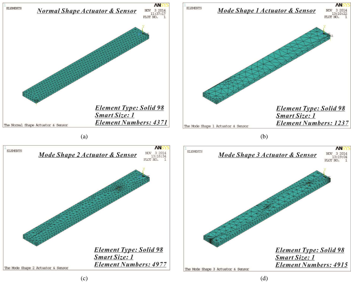
Figure 9. Meshing the mode shape and normal shape actuators and sensors. (a) The normal shape actuator and sensor; (b) The mode shape 1 actuator and sensor; (c) The mode shape 2 actuator and sensor; (d) The mode shape 3 actuator and sensor.
