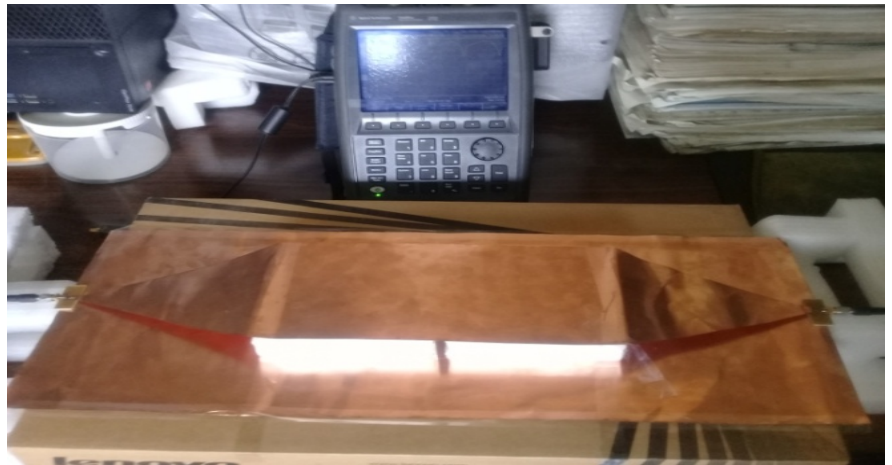
Figure 8. Fabricated TEM cell.
