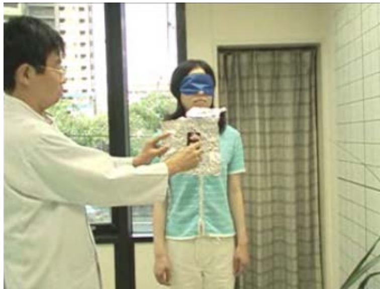
Figure 1. A cell phone was held about 1 m away from the blindfolded subject and aluminum foil was placed between the subject and a cell phone to shield the subject from the electromagnetic waves emitted by a cell phone. The subject's posture was normal.
