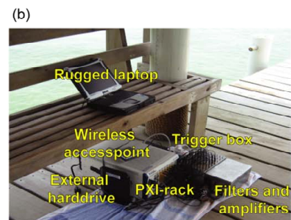
Figure 3. (a) Basic block diagram of the multi-channel data acquisition system; (b) Photo of the basic parts of the system (hydrophones omitted).
