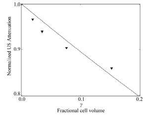
Figure 4. Experimental values of the normalized US attenuation in PVA-porcine liver cells composites with the best fit obtained for  $\eta_b/\eta_g = 6.54$  as a function of the fraction of the cell volume  $\gamma$ .
