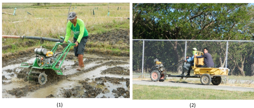
Figure 4. The two machines evaluated using the VFHBFI: 1) Micro-Tiller, and 2) Power-Tiller-Operated Hauler.
