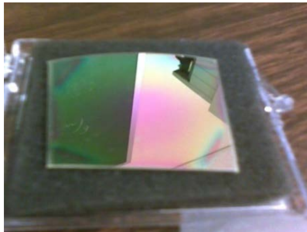
Figure 3. PLZT sample manufactured at the MEMS laboratory.
