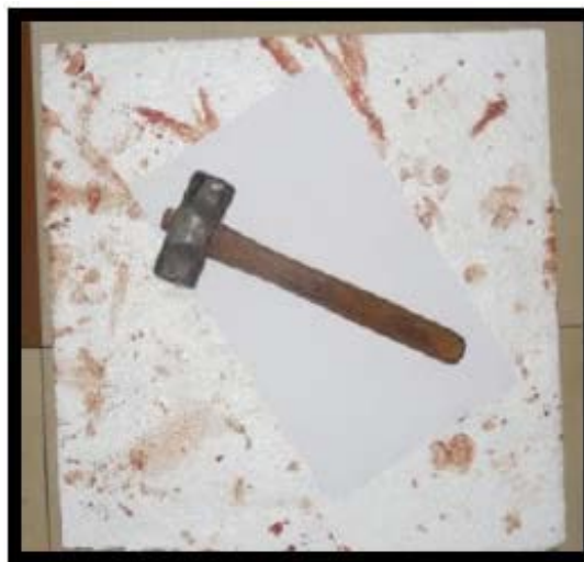
Figure 4. Thermocol sheet placed on the floor to avoid damage of the floor tiles. Paper sheet is placed on the thermocol sheet and hammer is dropped on the paper sheet by measuring the fall height from the top of the thermocol sheet.
